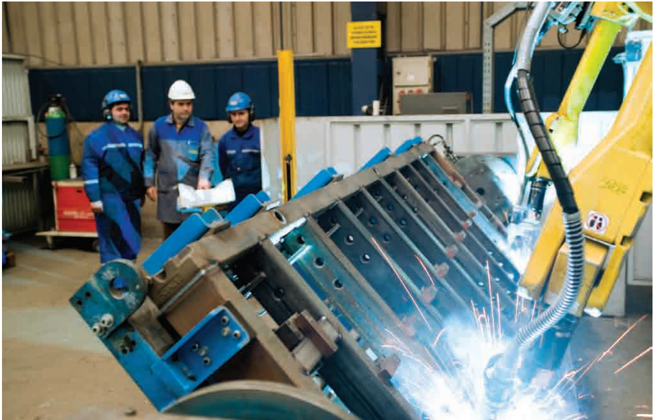
Fully Automated Fixtures and Robotic Welding has been applied for VINC'I production.
