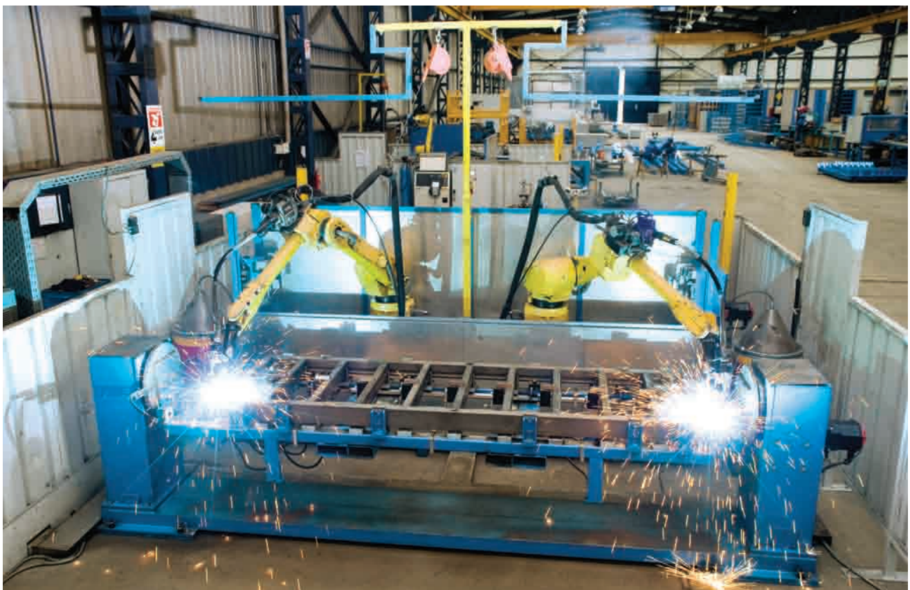
Fully Automated Fixtures and Robotic Welding has been applied for VINC'I production.
